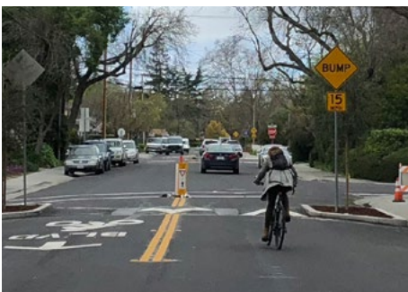
Speed cushions with curb extensions, Palo Alto, CA
